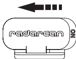
Fig. 1: Slide the switch to the left to turn on the PORTABLE MOSQUITO REPELLER.
