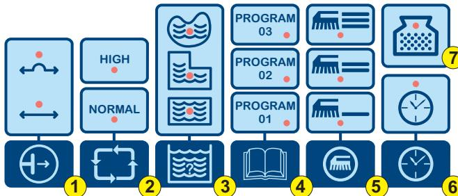
1. Auto detect: this feature prevents the robot from getting stuck on obstacles in the pool such as main drains, steps, ladders etc. Press this button to choose one of the following options:
