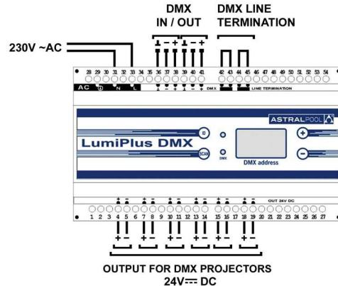
In installations with long lengths of power lines, it is recommended to install the Power Supplies as near of the projectors as possible (with a longer 230V~AC line).
