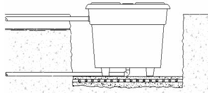
3.5.- Perforate the unit on the side where the electrical supply is to enter, with a diameter that matches the cable to be installed. Determine the section of the cable depending on power consumption and drops in voltage.
